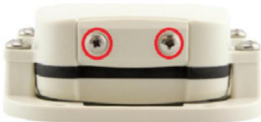
You will notice small text on the front where it says OFF. Once the front plastic piece is unscrewed, adjust the switch from the OFF position to the ON position. You will see that the device is now set to the ON position. The device is now on and will communicate three times a day, or your selected number if otherwise programmed, to the GPS platform.
