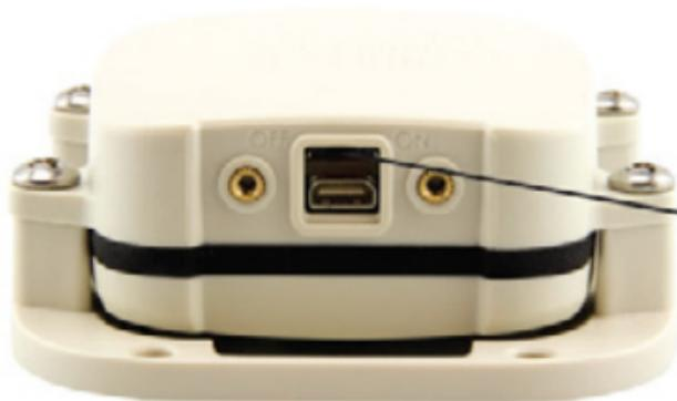
Remove cap and slide switch to turn on/off
