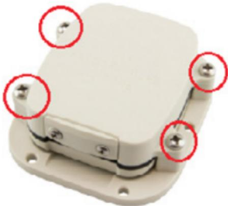
Gently remove the device from the plastic platform and flip it upside down. You will find four more screws. Unscrew them and remove the battery cover; you will find the four AAA batteries as shown below.
